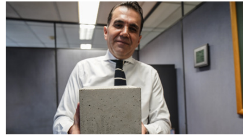
Carlos Castro holds a biocement brick — made exclusively from dried ash extracted from household wastewater. This could be a future market for the byproducts that come from Aguas Andinas' circular economy model.
